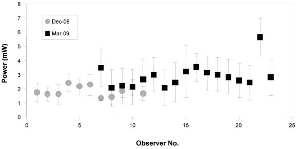
**FIGURE 1.**Output power (mW) required to see comfortably the beam of a GLP (532 nm) propagating through the atmosphere against the night sky background. Each point represents the average of the power readings for each observer; error bars represent 1 SD of the data.
