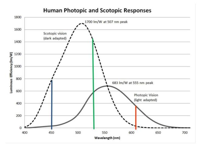
The hazard from flash blinding is substantially reduced when laser pointers emit red/orange wavelengths at 615 nm or longer. The hazard from laser aircraft illuminations would be effectively eliminated if green and blue laser pointers were not available. Colors at 615 nm and longer, viewed with night adapted vision, are only 1.4% as bright appearing as green at the commonly manufactured 532 nm wavelength.
